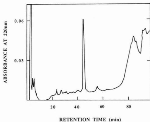
FIG. 4. Separation by high performance liquid chromatography of the peptides generated by CNBr digestion of human MGP. Separation of 20  $\mu$ g of the cyanogen bromide digest of human MGP on a Vydac reverse-phase C-4 column (4.5  $\times$  250 mm). Buffers and gradient are described in the Fig. 2 legend.
